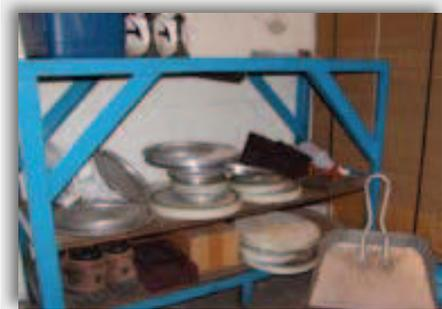
*BEFORE. Machine parts are all stored in an unorganized stack. Two pieces needed for a particular job are almost never found together.*
