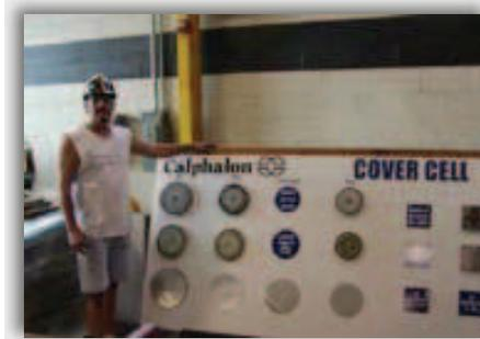
*AFTER. Tool shadows are used to organize all the parts so it's impossible to make mistakes during setups.*
