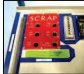
This scrap separator solution began as six styrofoam cups that the assembly operator taped together so she could sort defects into groups as she found them.
