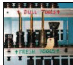
In this cell, operators leave dull tools in the red location on the machine face and maintenance returns them, sharpened, to the green location.
